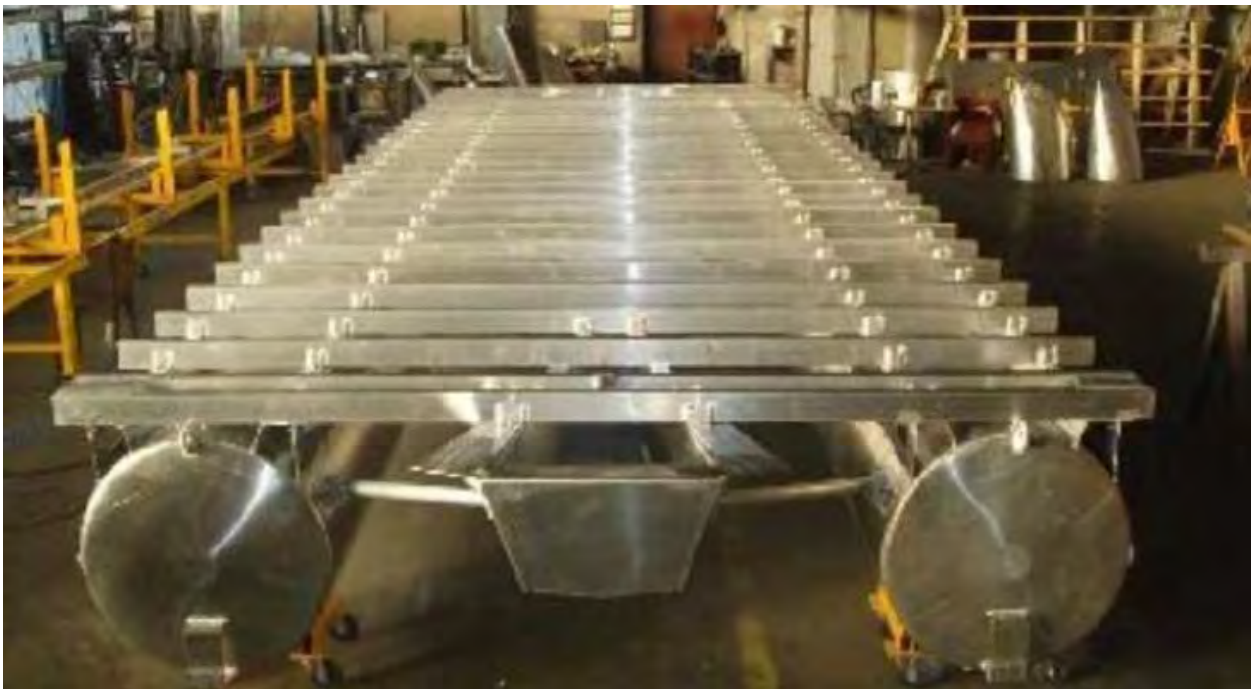
Figure 3. Pontoon sled for transporting the GeoProbe coring machinery.
