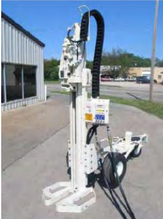
Figure 4. GeoProbe ® 540MT which will be used for coring.
