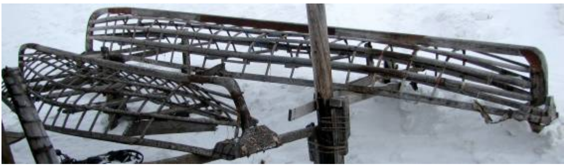
Skin-boats are stored on racks. These two need new frames.
