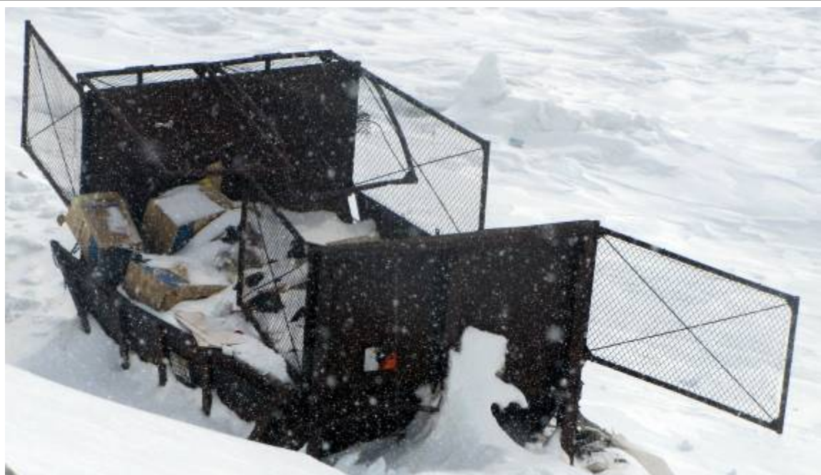
Diomedede's incinerator was damaged during a storm-surge.
