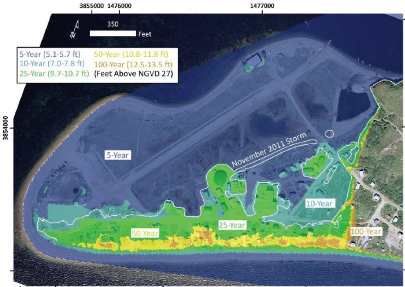
Below: Flooding projections for Golovin Spit based on measurements and numerical modeling (Smith 2014)
