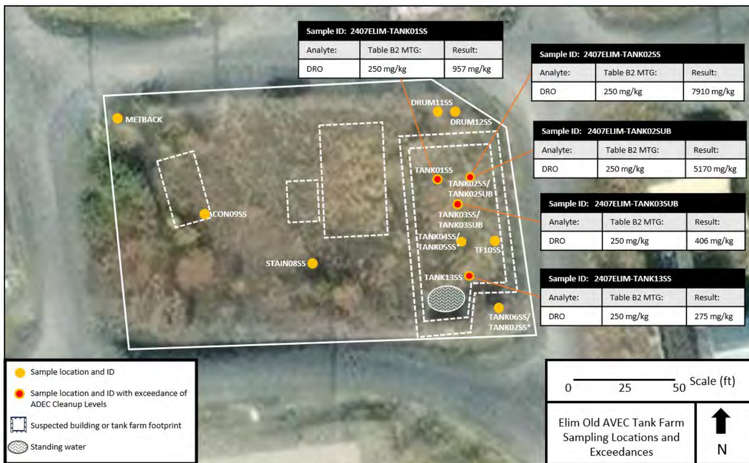
Figure 3 Elim Old AVEC Tank Farm sampling locations and exceedances.
